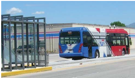
MAX BRT vehicle with three boarding doors, Salt Lake City, UT
